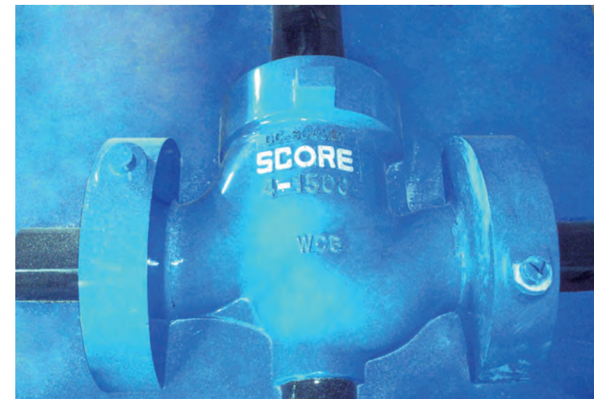
Finished Wooden Pattern of GC100 4"-1500# Body
